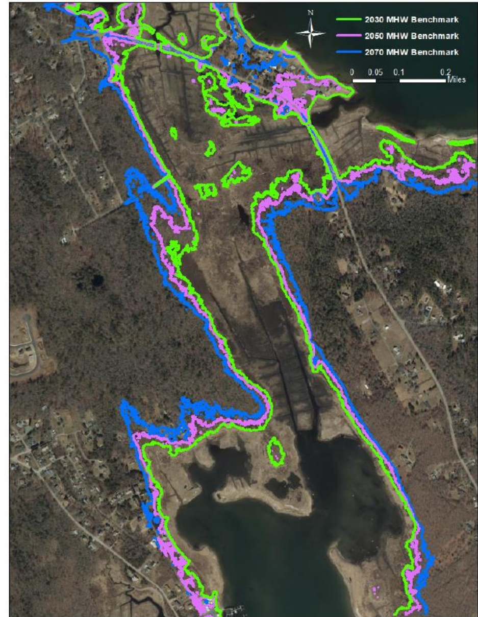
Figure 2. Mean High Water benchmark under 2030, 2050, and 2070 sea level rise scenarios, from the MC-FRM.
